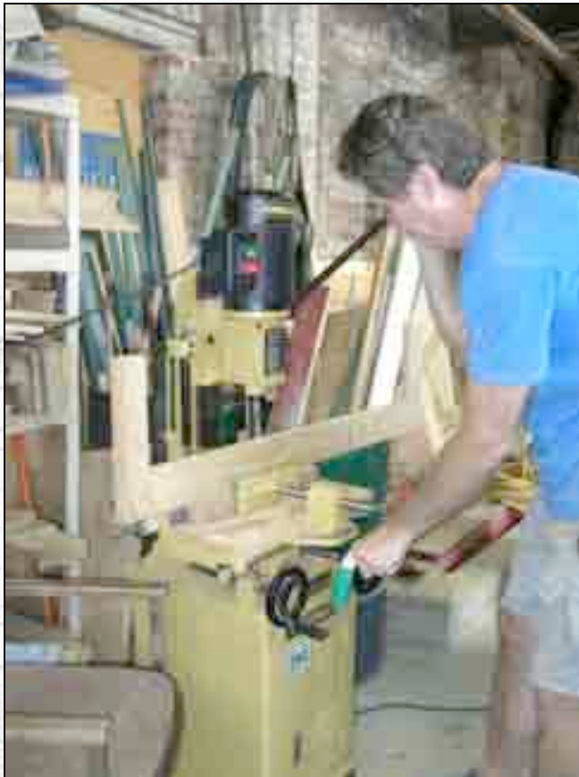
Don uses a mortis drill to insert mortises into a window frame.
