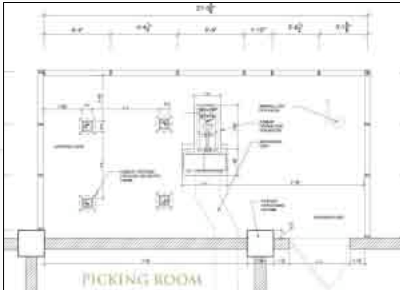
Floor plan showing location of dust collector in the basement of the Paint Shop.
