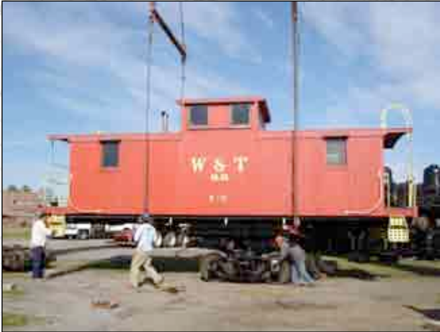
View of caboose being hoisted onto railcar trucks.
