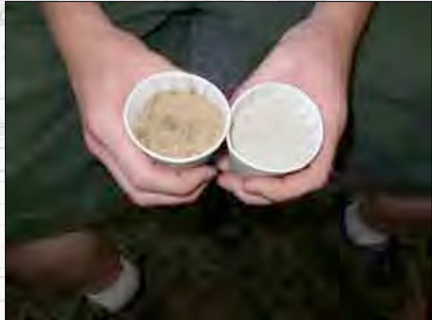
The mortar analysis shows that Savannah River sand (left) was historically used on most of the buildings in the repair shops complex; however, a finer sand with less color was originally used on the passenger station.
